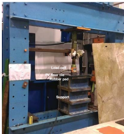
Figure 11 Compressive strength and durability test of PV floor tile
