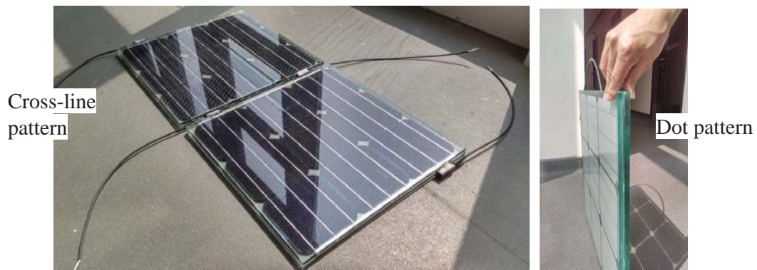
Figure 5 PV floor tiles with different anti-slip surfaces
